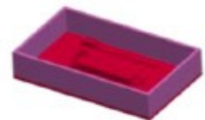
Place flask over drag portion of the pattern
