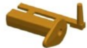
Shakeout mold and trim off gating system
