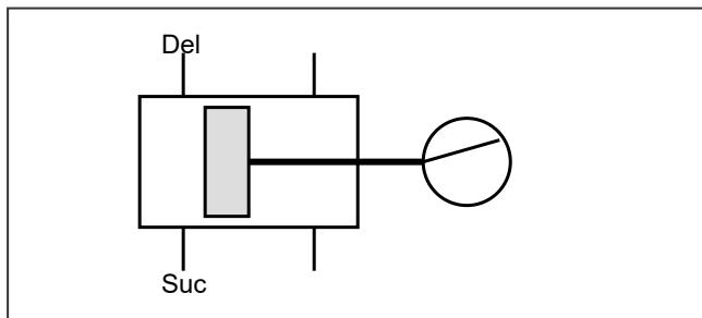
**Q.6. (b) [Theory]** What is an **Indicator Diagram**? Draw the theoretical and actual indicator diagrams for a reciprocating pump showing the effect of acceleration head. [7]
