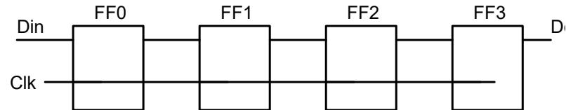
Figure: 4-bit SISO Shift Register
