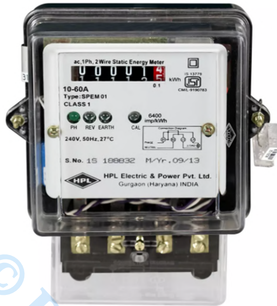
Figure 19. Energy Meter (example of integrating instrument)
