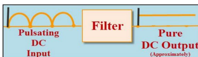
Smoothing Filter to obtain Pure DC
