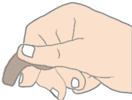
Gently press the ball of soil over the forefinger with the thumb, and extrude it in length to form a hanging ribbon
