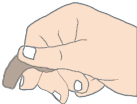
Gently press the ball of soil over the forefinger with the thumb, and extrude it in length to form a hanging ribbon
