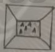
sloped footing or foundation
